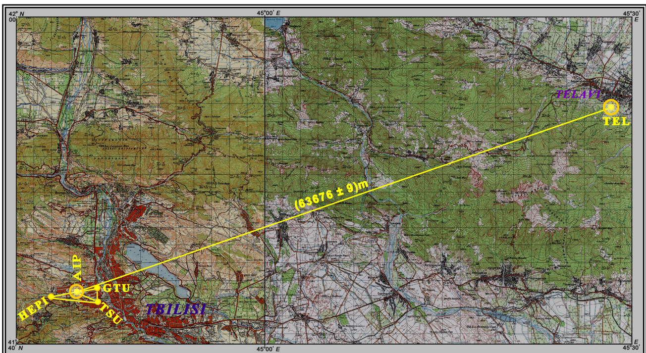
Figure 1. Disposition of EAS goniometers of the GELATICA network Sensitivity circles are shown for AIP and TEL goniometers for vertical showers only for showers with maximal energy E = 10^{20} eV;
