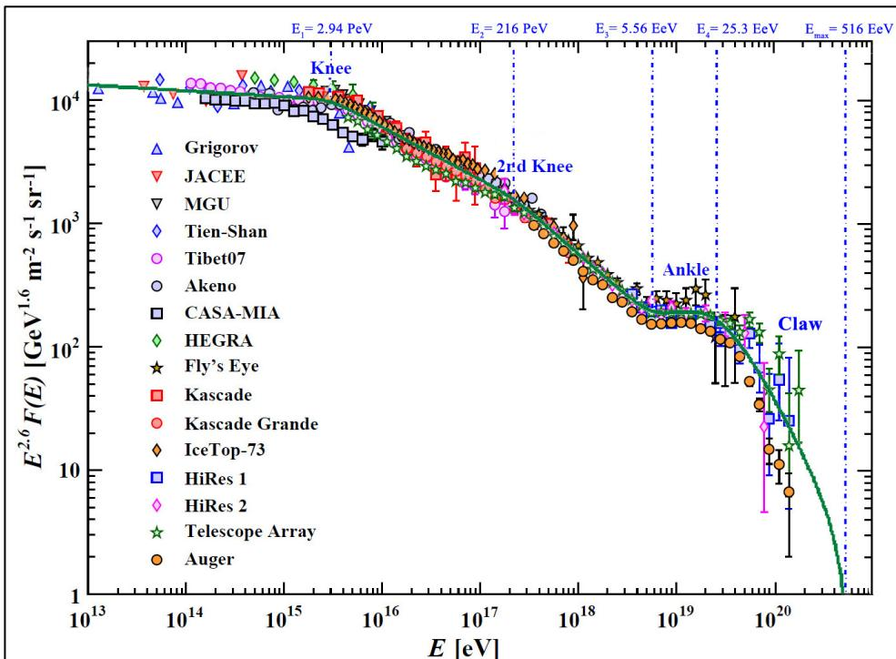
The EAS energy spectrum is shown as a function of energy-per-nucleus from air shower measurements. Every flux value is multiplied by the correspondent energy in the power 2.6. The green line represents the spectrum function defined above.
